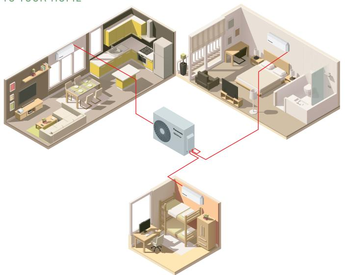
Panasonic Multi TZ systems provides comfort up to 3 rooms or spaces at home. Using one compact single unit for connecting from 2 up to 3 indoor units is saving space outside. Each room will have independent control, enjoying more precise temperature control and saving energy when room is not in use. Quiet and compact styled indoor unit will fit easily in any indoor space, achieving energy rank of A++ in cooling and A+ in heating.
